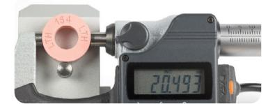
The "T"'s impressed in the ring should be placed exactly on the indentation of the micrometer.
